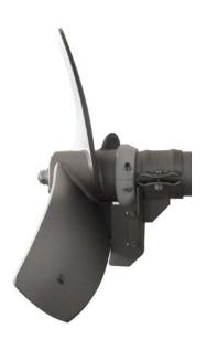
POM protective sleeve to minimize abrasion. the protective sleeve is suitable for many long axis agitators or submersible motors of SUMA. It can be retrofit on installed agitators. It is mountable with just few work steps. The installation instruction is within the delivery scope.
